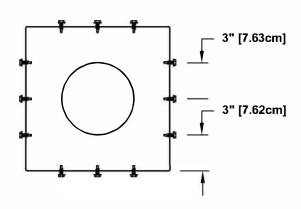
Roof Vent with Curb Mount Flange accessory installed onto roof curb.
