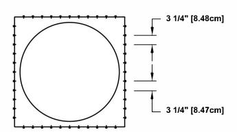
Roof Vent with Curb Mount Flange accessory installed onto roof curb.
