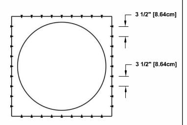
Roof Vent with Curb Mount Flange accessory installed onto roof curb.
