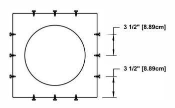
Roof Vent with Curb Mount Flange accessory installed onto roof curb.
