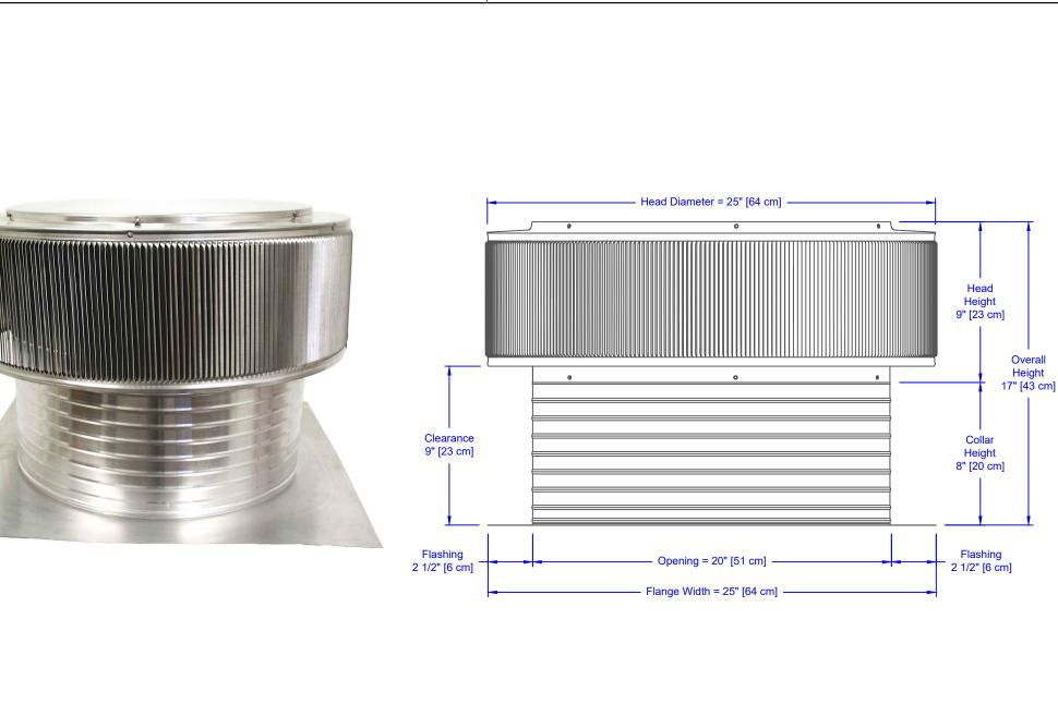
All Aluminum ConstructionMinimum Thickness = 0.040" [1.02 mm]
